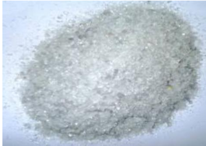
Figure 10. Glass wastes from Addis Ababa as fine aggregate
