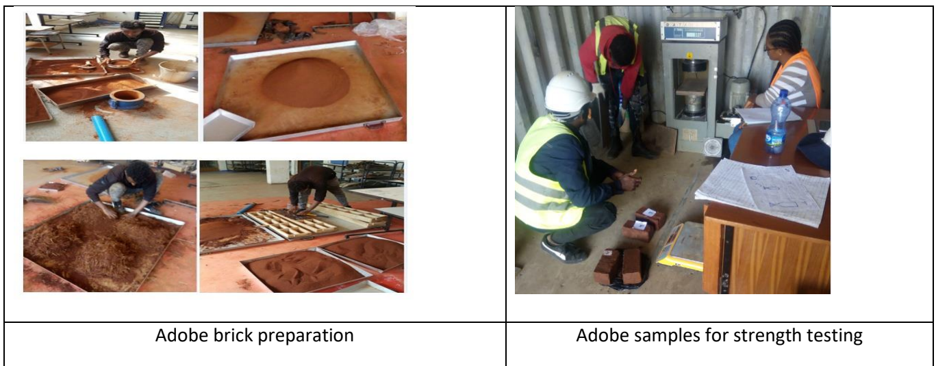
Figure 6. Adobe brick sample preparation and testing
