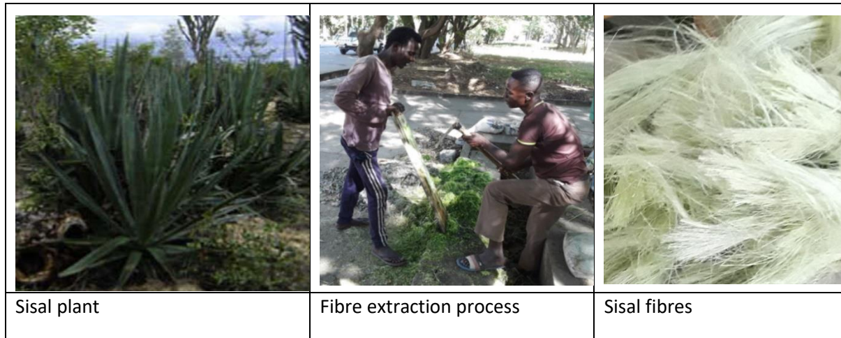
Figure 9. Sisal fibre a natural fibre for arresting tensile cracks in concrete
