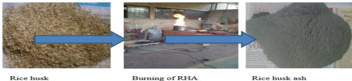
Figure 7. Rice Husk Ash an alternative cementing material
