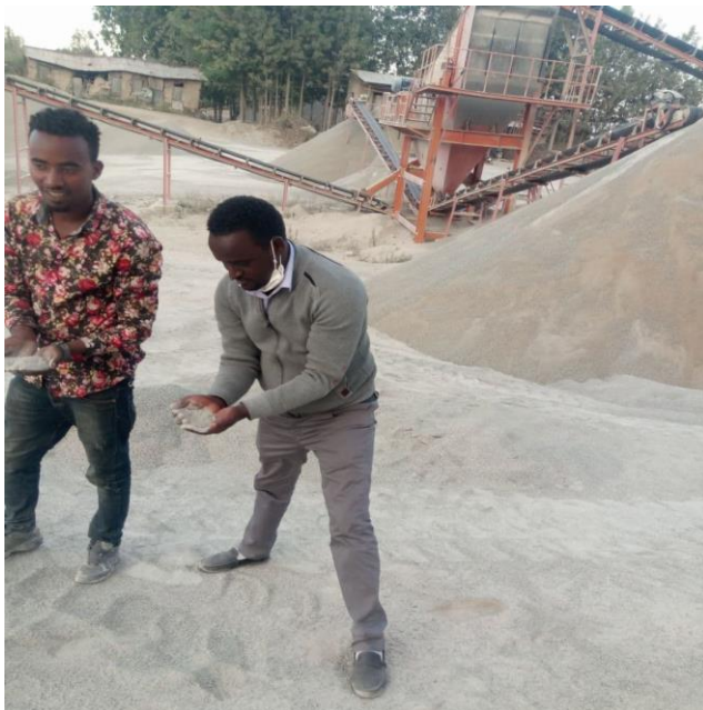
Figure 11. Crusher dusts from Hawassa Monopol as fine aggregate
